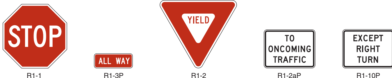
Figure 2B-1. STOP and YIELD Signs and Plaques
