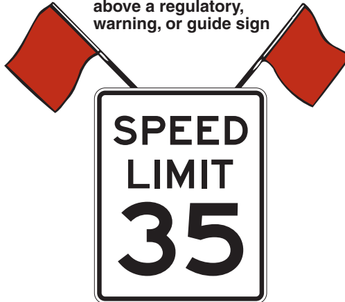
Figure 2A-1. Examples of Enhanced Conspicuity for Signs
