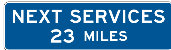
Figure 2I-2. Example of Next Services Plaque
